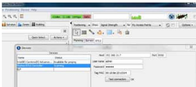
To activate a device for scanning, the device must first be "connected" to the laptop. This can be a NIC card installed on the laptop, Ekahau RTLS Controller, or a tag connected to the survey in "survey mode". Connected devices will be displayed in the "Devices" list. Simply select the desired device and select "Use for Scanning".
